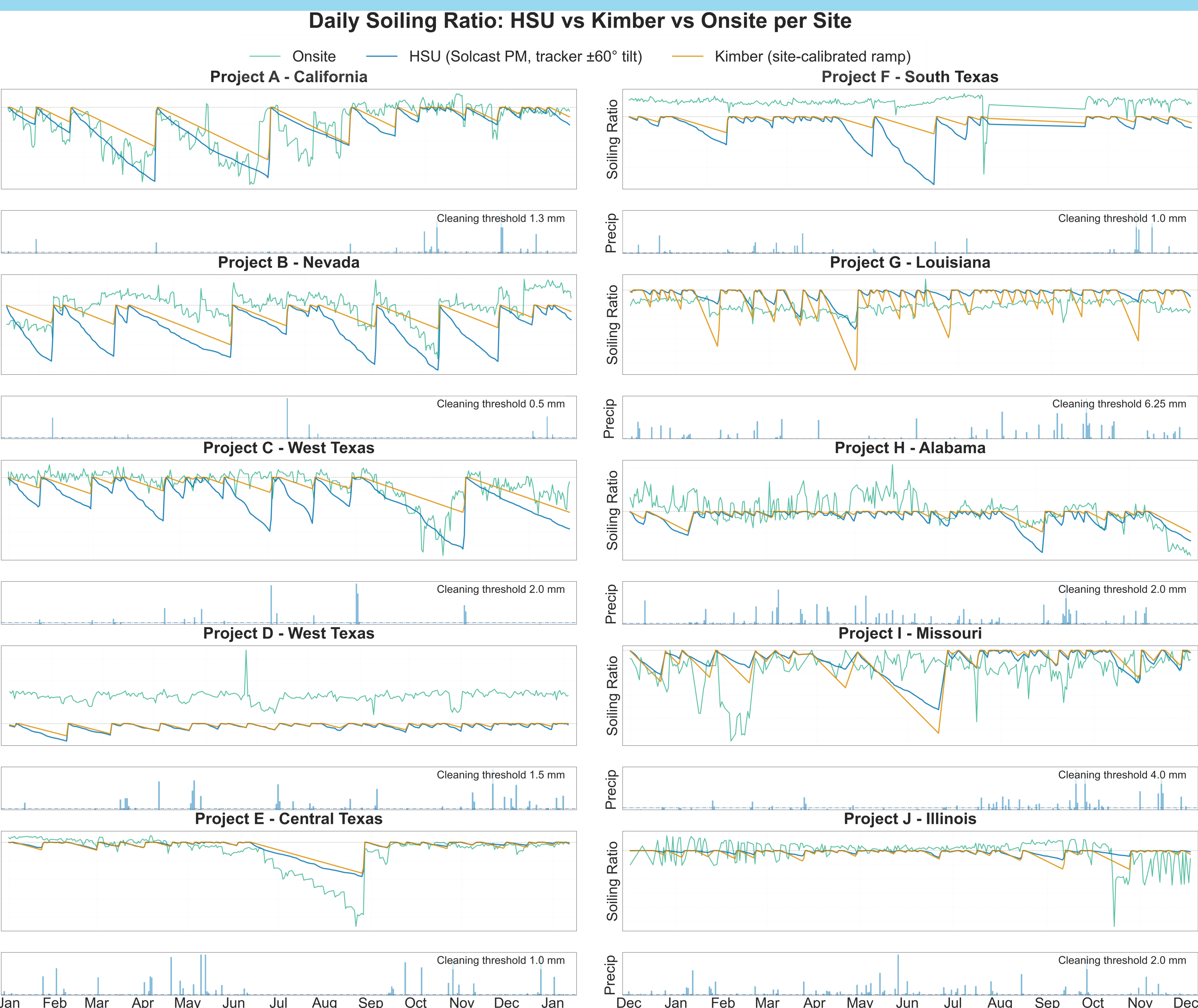
Figure 1: Daily dust soiling profile from the measured soiling experiment (green) and the results from the Kimber and HSU models (orange and blue, respectively).
