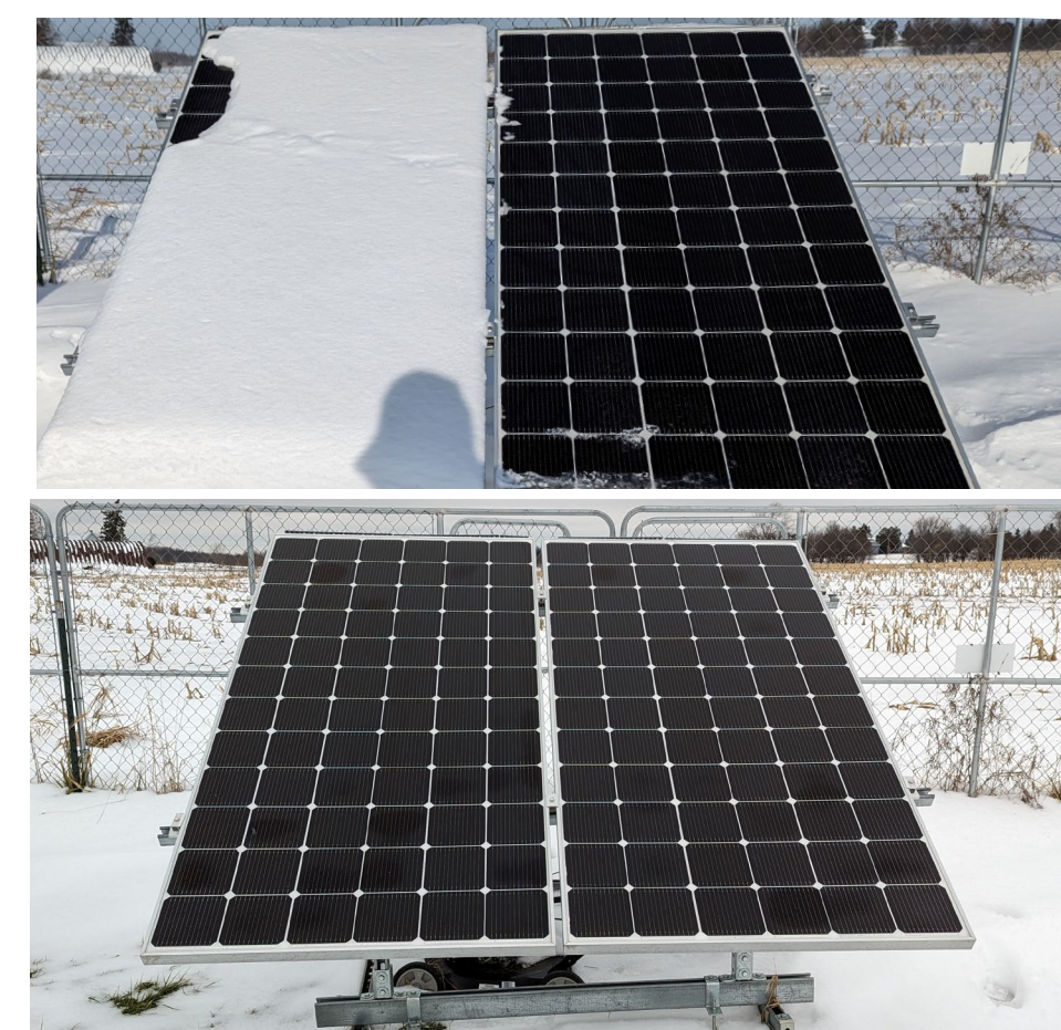
Figure 4. Photographs of soiling kit modules. Soiled module on left side. Cleaned on right side.
