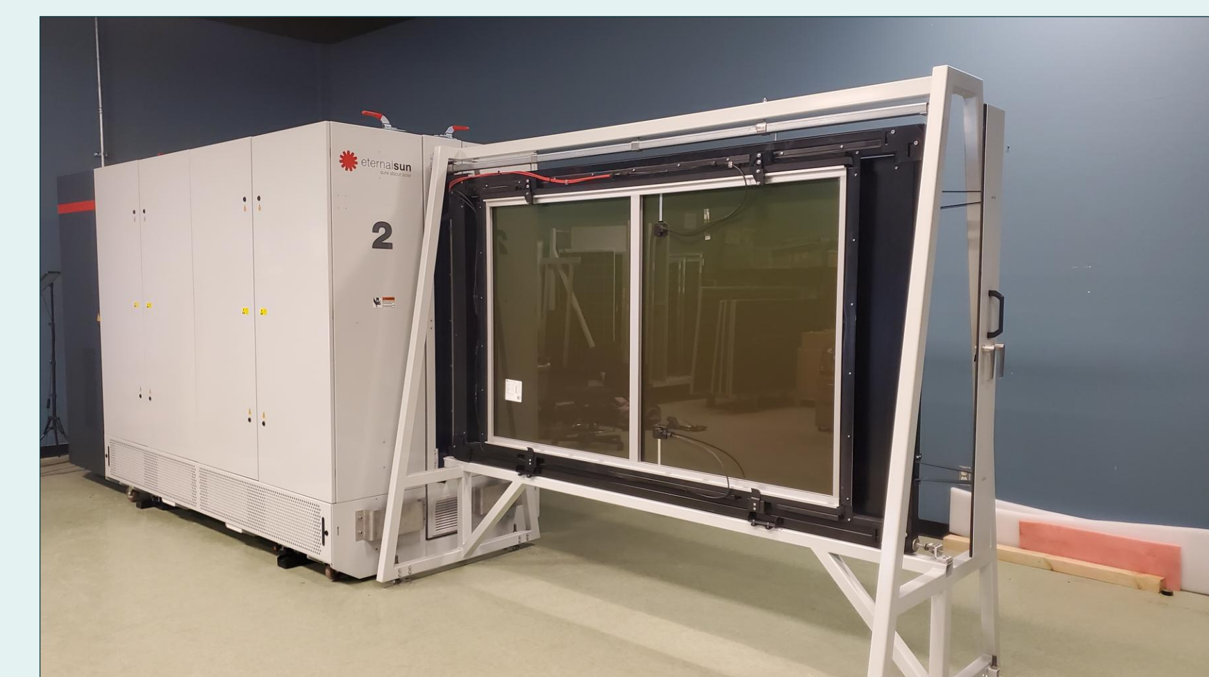
Fig. 2a: Eternal Sun LED solar simulator (enclosed closed chamber, dual-side capable).
