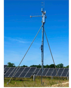
Figure 1: Quanterra Systems eddy covariance flux tower at the Bancroft Station agrivoltaic array.
