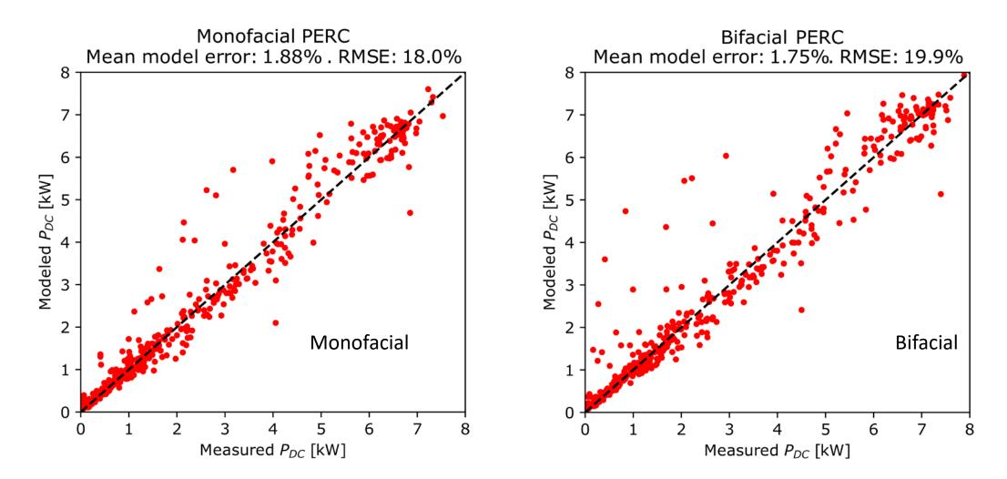
\*SAM v2018.11 using 15-minute measured DNI, DHI, albedo from SRRL BMS. Andreas, A.; Stoffel, T.; (1981). NREL Solar Radiation Research Laboratory (SRRL): Baseline Measurement System (BMS); Golden, Colorado (Data); NREL Report No. DA-5500-56488. Bifacial systems assume 5% shading loss, 5% mismatch loss, 0% transmission factor
