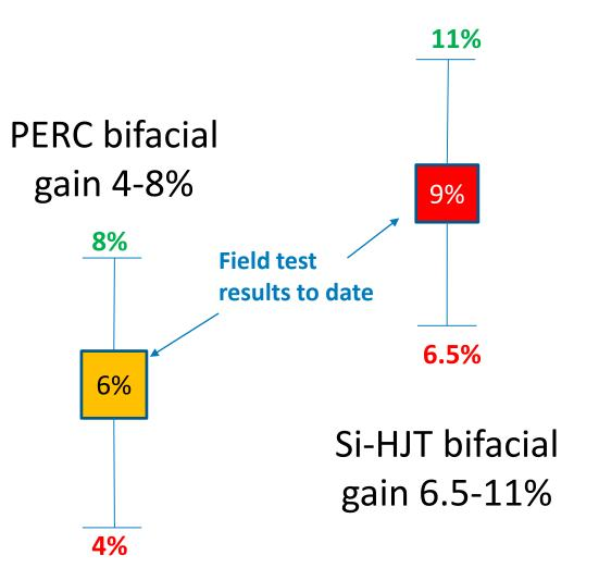
\*SAM v2018.11 using 15-minute measured DNI, DHI, albedo from SRRL BMS. Andreas, A.; Stoffel, T.; (1981). NREL Solar Radiation Research Laboratory (SRRL): Baseline Measurement System (BMS); Golden, Colorado (Data); NREL Report No. DA-5500-56488. Bifacial systems assume 5% shading loss, 5% mismatch loss, 0% transmission factor
