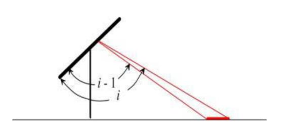
$$G_{rear} = G_{DNI,rear} + \sum_{i=1^{\circ}}^{180^{\circ}} VF_{i} \cdot F_{i} \cdot G_{i} ;$$
