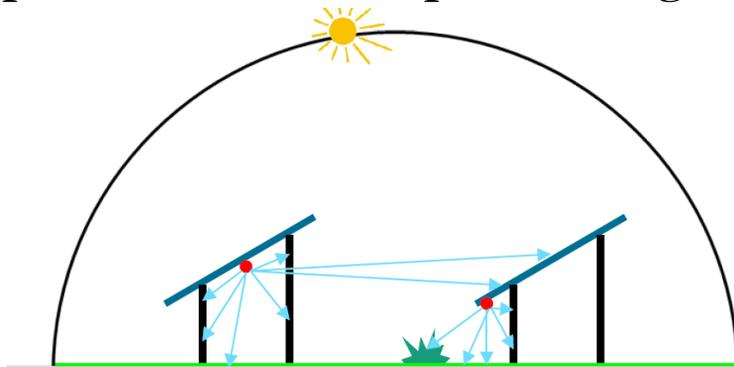
1. Rays are traced in all directions from sensor points. The sky dome is a heterogeneous light source.
