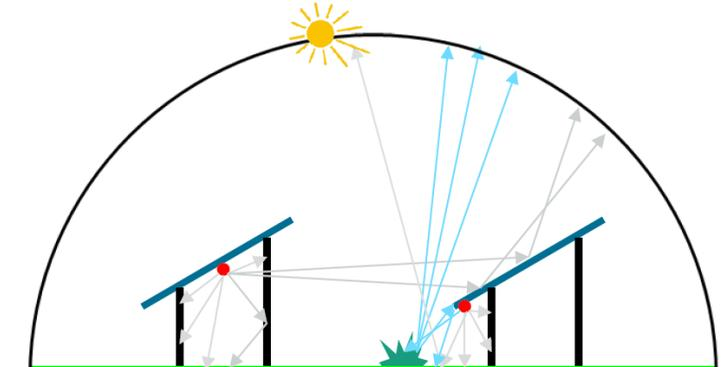
3. Light reaching sensor points is calculated by adding up all the rays that reach the sky and considering losses from absorption.
