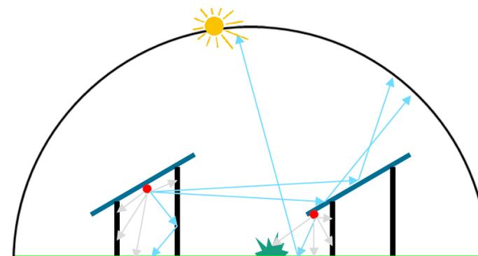
2. Rays bounce off surfaces. Specular and diffuse reflections are considered. Multiple bounces are allowed.
