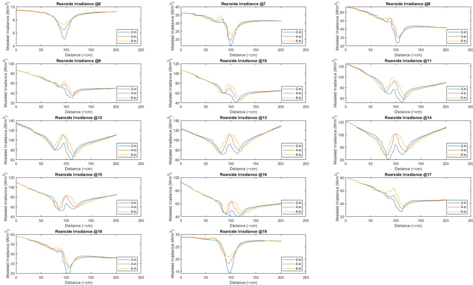
Moving torque tube further from module increases irradiance directly behind but decreases irradiance further away.
