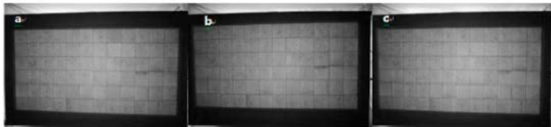
Fig. 2. EL image of double glass module after DH test. (a) DH1000h; (b) DH2000h; (c) DH3000h.
