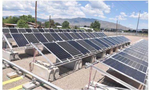
Fig. 1. Sandia’s 4-tilt test bed. Rows are tilted between 15 and 45 degrees with rear irradiance sensors at the top and bottom of each row, near the center of the row.
