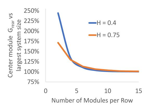
Within a distance of 5 m from the row edge, rear irradiance and  $BG_E$  is increased by 25% on the south edge, and 10% on the north edge.
