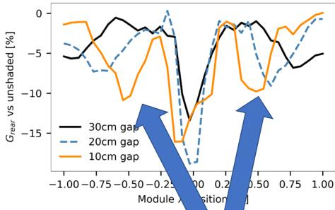
As expected, there is a primary peak in shading loss directly behind the tube at X = 0 m, reducing  $G_{rear}$  by 15% - 20%.
