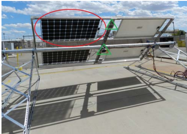
Fig. 7. Bifacial PV module under test circled in red. Top and middle rear-facing reference cells indicated by green triangles. View is to the south.
