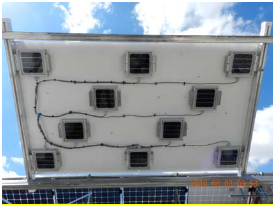
Fig. 11. Sandia's high spatial resolution rear irradiance module blank with ten reference cells measuring rear irradiance, used for validation of the irradiance model.
