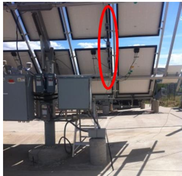
Fig. 1. Back surface irradiance measurement locations on the NREL array.
