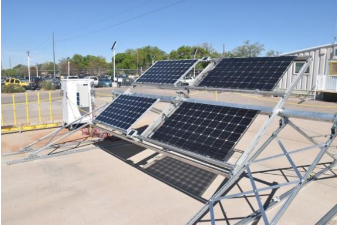
Fig. 3. Bifacial modules (right) on test rack at Sandia National Laboratories.
