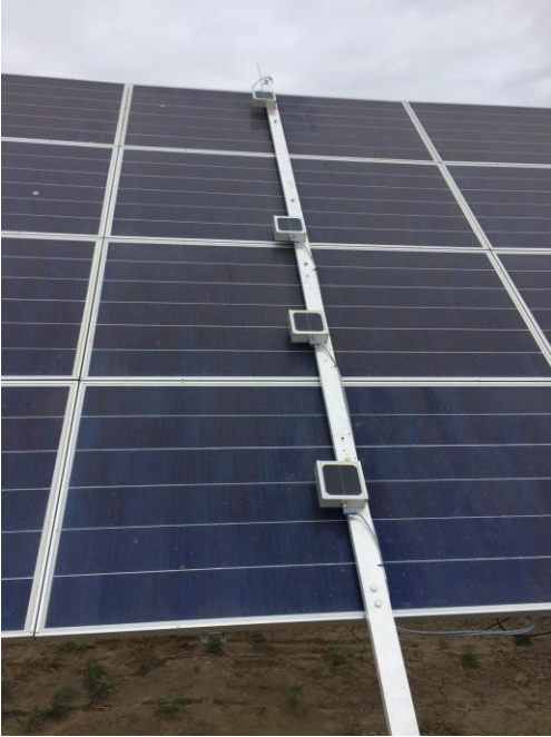
Fig. 8. Picture showing the setup of reference cells installed along the width of the west single-axis tracker at the SunPower R&D Ranch in California.
