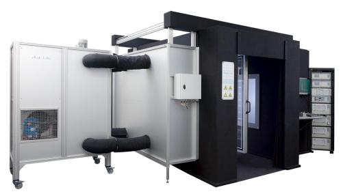
Fig. 4.3.1 Class AAA solar simulator from h.a.l.m. used at CFV
