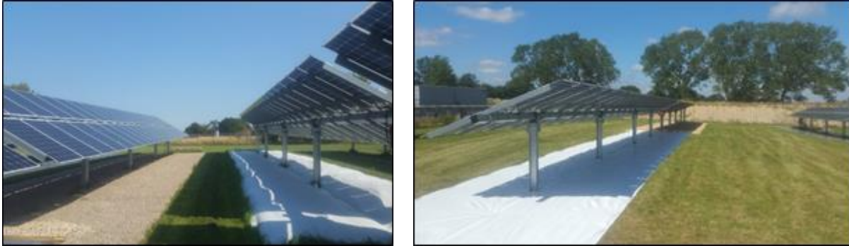
Figure 101: Ground cover (albedo) experiments on fixed-tilt strings (left) and equivalent experiments on HSAT strings (right).
