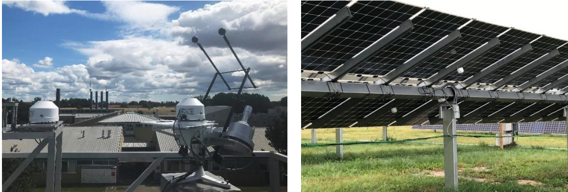
Figure 103: (left) Direct normal, diffuse horizontal, and global horizontal radiation measured at the campus solar radiation monitoring station. (right) Spectrally flat class C pyranometers installed on the backside of a fixed tilt array T11.
