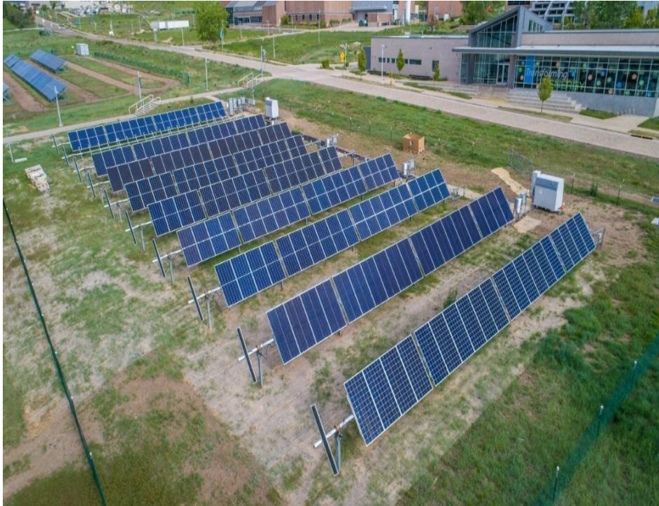
Figure 88: 1-axis tracker testbed for the NREL bifacial module and system performance monitoring project.
