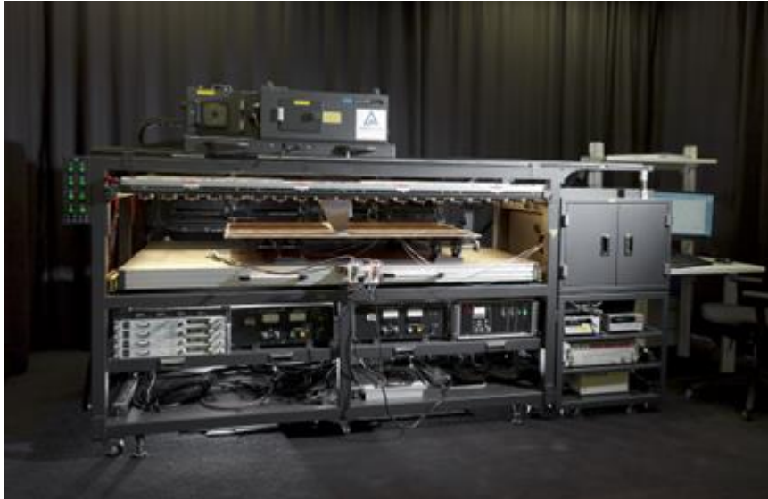
Figure 10: System for spectral response measurements of full-size PV modules (Source: TÜV Rheinland Group).
