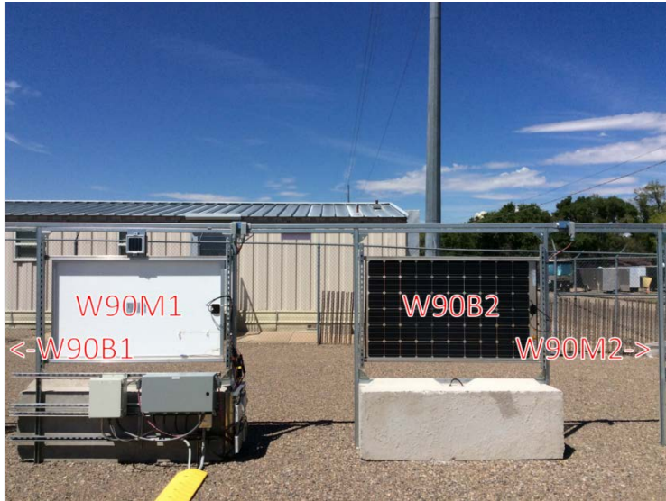
Figure 13: Photograph of W90 modules, looking west. Modules W90M1 (left) and W90B2 (right) are visible, while modules W90B1 (far left) and W90M2 (far right) are out of the picture. The power pole that casts a shadow on the W90 modules when the sun is near a west azimuth can be seen directly behind module W90B2.
