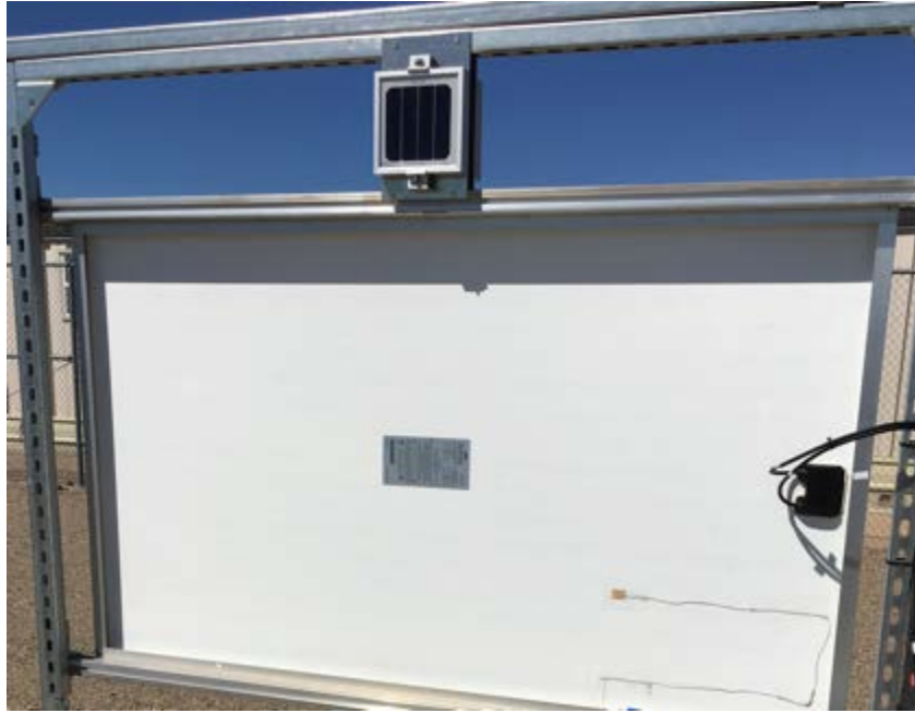
Figure 3: POA reference cell (top center of picture) mounted to measure backside irradiance, shown here for one of the monofacial modules in the W90 orientation. Also visible in the lower right is the yellow thermocouple measuring module temperature.
