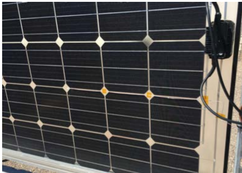
Figure 2: Backside of Prism module showing location of yellow thermocouples.
