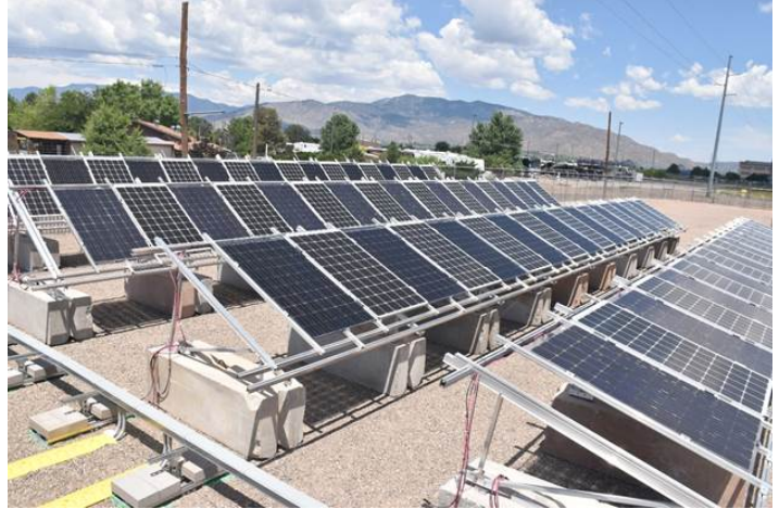
Fig. 3. Fixed-tilt, string level bifacial testbed at Sandia.
