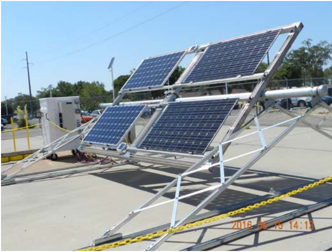
Fig 1. Sandia’s adjustable, single modules IV curve rack in Albuquerque, NM. Two bifacial modules are on the right and two monofacial modules are on the left.
