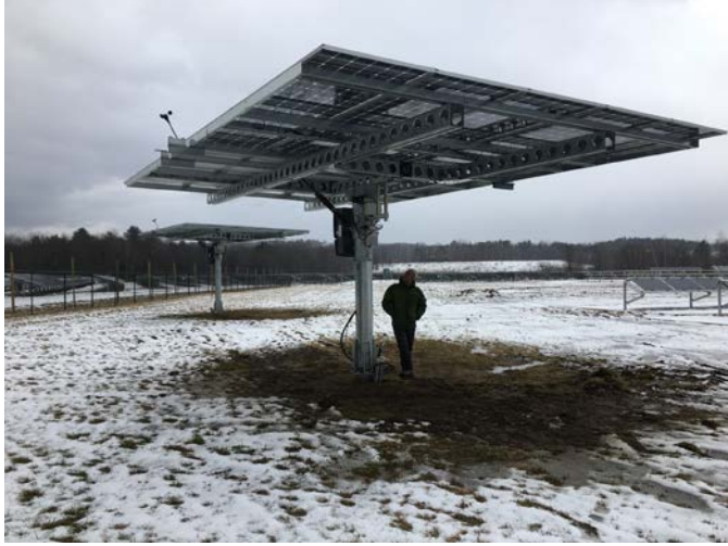
Fig. 5. Two-axis trackers with bifacial modules at the Vermont Regional Test Center.
