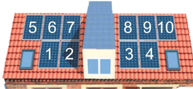
Figure 11: Simulated system with the PV module placement on the roof with a dormer [20].
