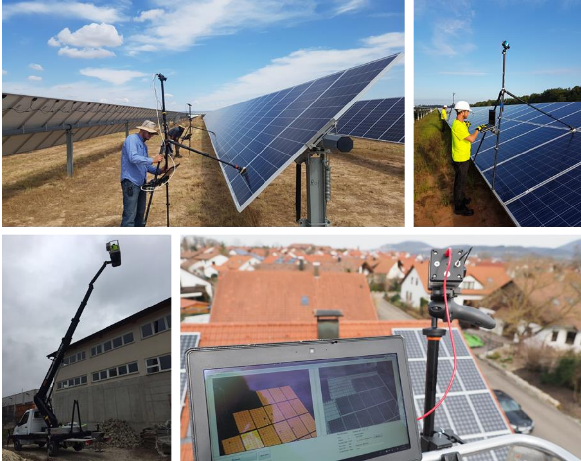
Figure 95: Field application of the DaySy system with full PV string biasing: Top: Multiple cameras inspect the same PV string at the same time for increased throughput (Source: Solarzentrum Stuttgart GmbH). Bottom: Hail-screening from an aerial platform [147].
