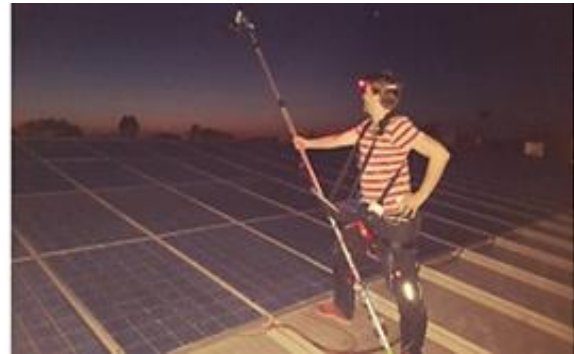
Figure 50: Handheld EL imaging system [86].
