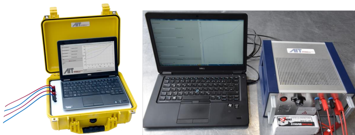
Figure 22: A battery powered dark I-V measurement system suitable for outdoor PV module evaluations produced by “AIT”. On the right, the previous prototype.
