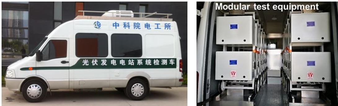
Figure 29: PV plant testing vehicle in China.
