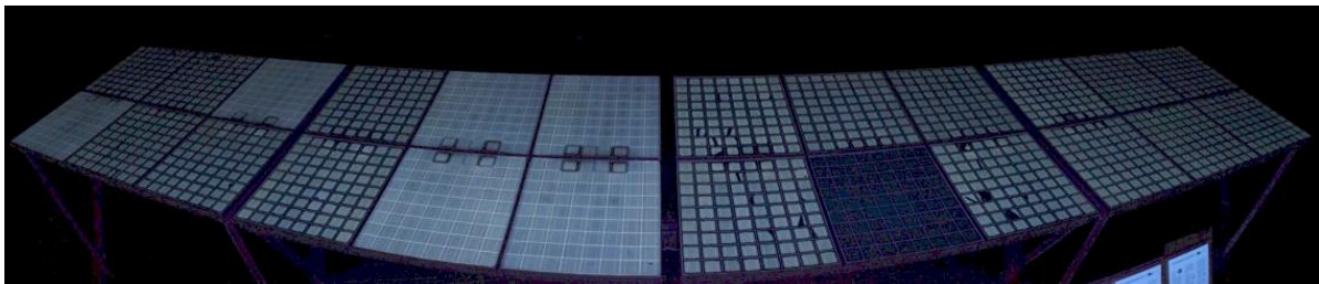
Figure 86: The image stitched from 10 single images taken at ISO3200, 1/5s, f2.0 from a distance of 5 m in the centre to 8 m to the farthest PV module. Note the fainting fluorescence due to less excitation at greater distances and flatter radiating angle.
