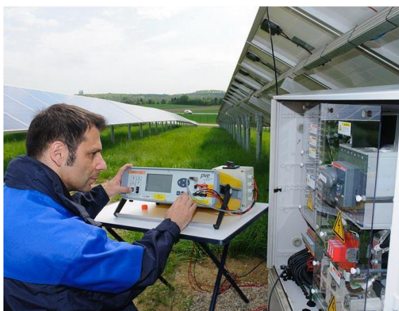
Figure 9: Typical test set up for I-V curve measurement of PV string in the presence of field combiner boxes. The DC input of the inverter and string fuses must be disconnected to make PV string terminals accessible (Photo: TÜV Rheinland).
