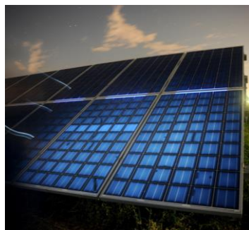
Figure 84: UVF image, left with urban stray light in a large city and right with good contrast in a darker environment.
