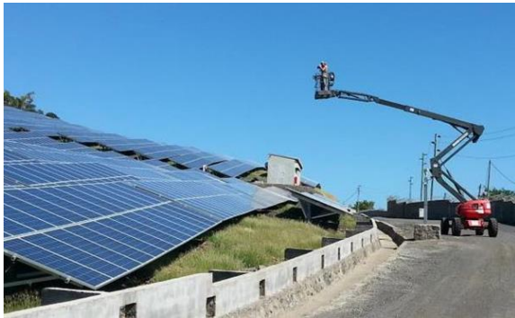
Figure 49: Mobile outdoor imaging system based on cherry picker [85].
