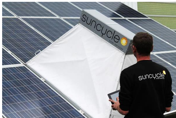
Figure 52: CTU Flex EL system by SunCycle (image from suncycle.eu) [106].
