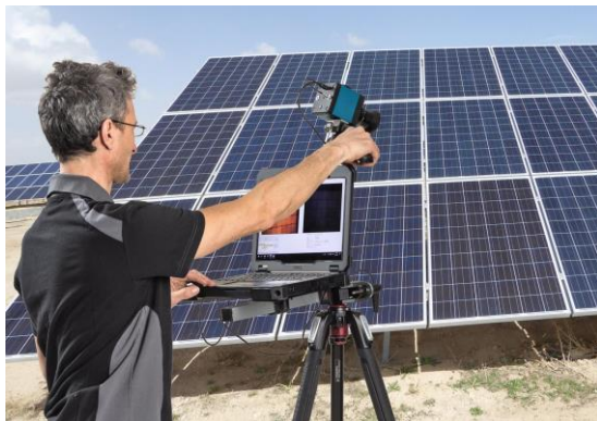
Figure 45: Application of daylight EL camera (copyright Fraunhofer ISE).
