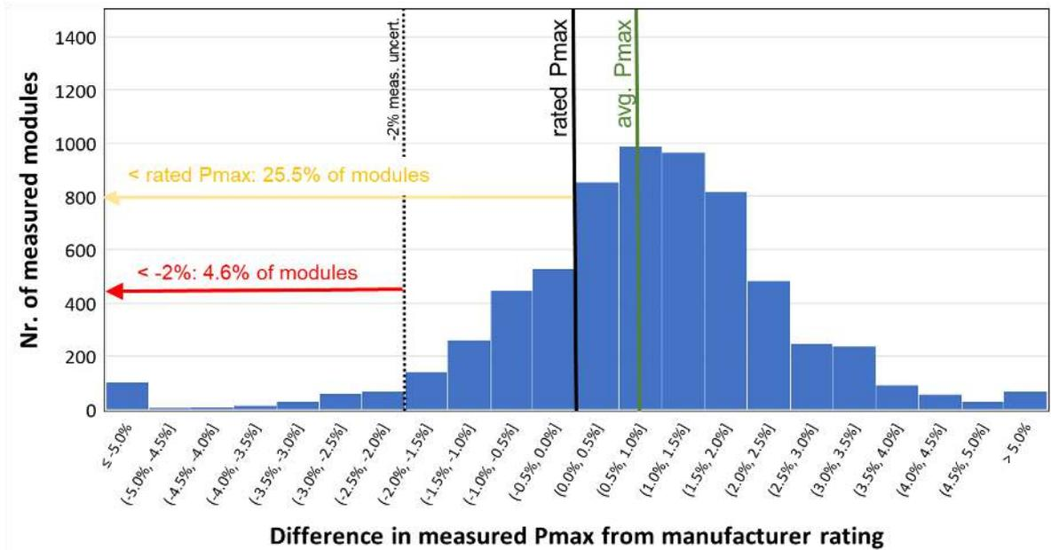
Statistical analysis done by Eternalsun on around 6500 new modules with 96 different PV module types from 29 different manufacturers. [35] Considering the measurement uncertainty of +/-2% a total of 4.6% of the modules are below the gate 1 limit defined by the IEC 61215 standard. [IEC 61215-1:2021]
