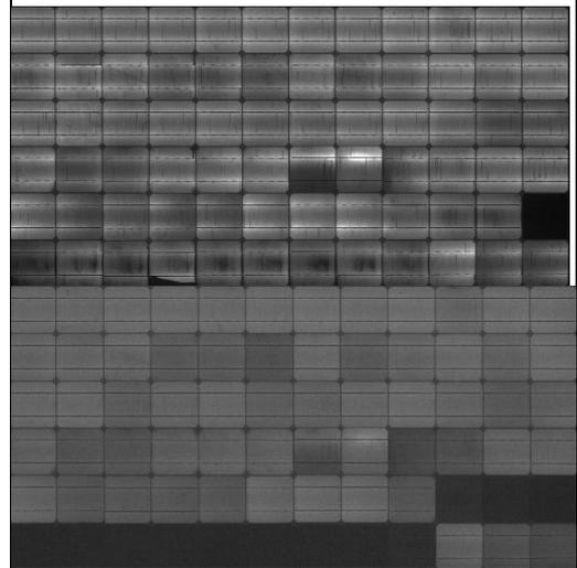
PID affected module with power loss of 89%, left: EL at 1.5 x  $I_{sc}$ , right: I-V curve of the same module at 1000 and 200 W/m<sup>2</sup>. [35]
