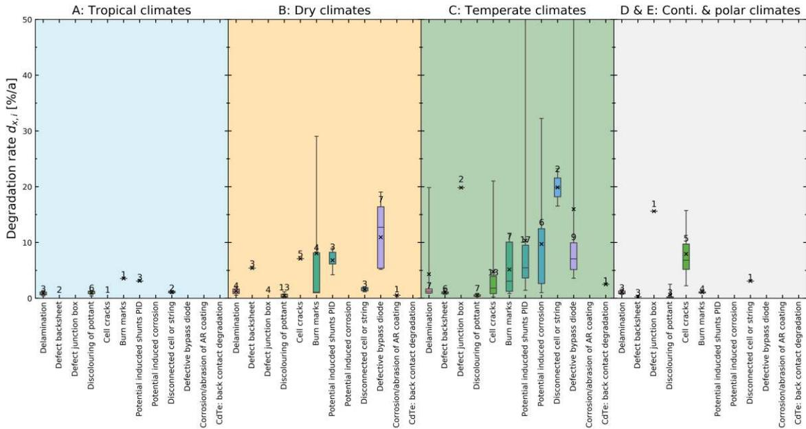
Figure 15: Box plot of degradation rates  $d_x$  of PV module affected by failures  $x$  sorted by climatic zones. The numbers show the quantity of data per failure in the database. The cross shows the mean degradation rate. The boxes include 50% of all values, the whisker show the full range of existing values. The middle line in the box shows the median.
