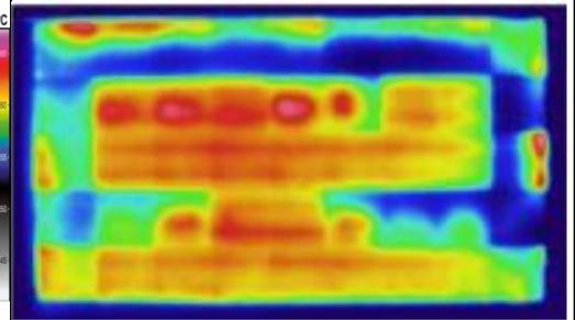
Strings with PID, detected with IR thermography. [16]
