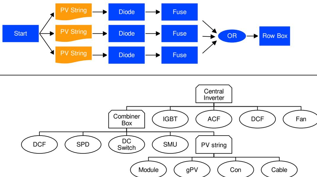
Figure 5: Examples of Reliability Block Diagram (TOP) and Fault Tree (BOTTOM). Adapted from [11].
