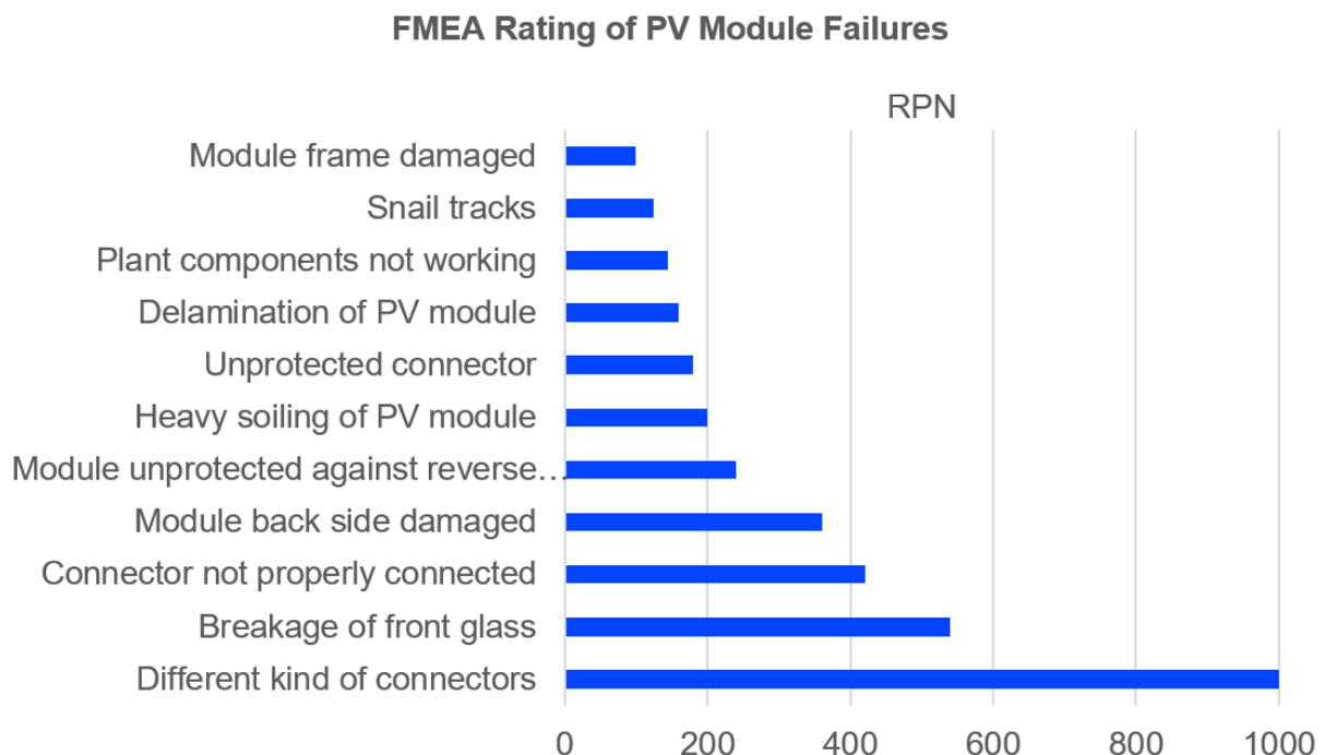
**Figure 2: Example of rating of PV module failures based on classic FMEA. The rating of the technical risks was based on the statistics of failure reports from TÜV Rheinland. RPN is the product of S, O and D where each factor is an integer between 0 and 10 [2].**
