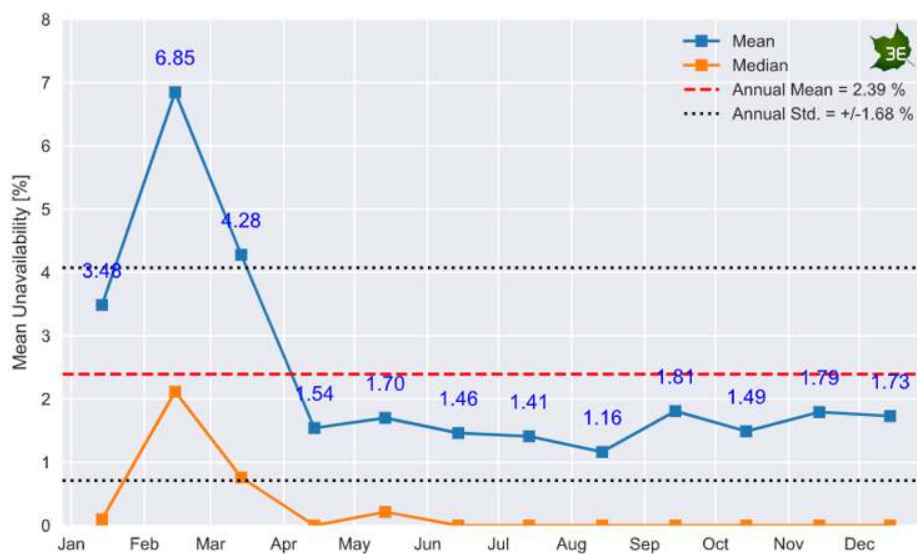
Figure 14: Statistical indicators of mean monthly unavailability of 533 PV plants in 2019 (majority installed in Belgium, Germany and Switzerland)
