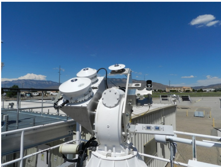
Figure 1 Two-axis tracker with pair of spectroradiometers (left) at the PSEL facility.
