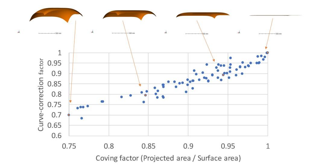
Parameters of the curves were given by random numbers. Curve correction factor was calculated by the ray-tracing simulation using 1E8 rays distributing by the direction weighted by the annual distribution of the incident angle on the horizontal plane.
