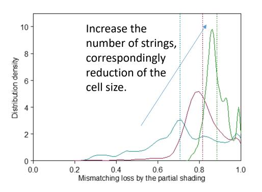
The ratio of the power output of the partially shaded module is less than the ratio of the area in the sun.
