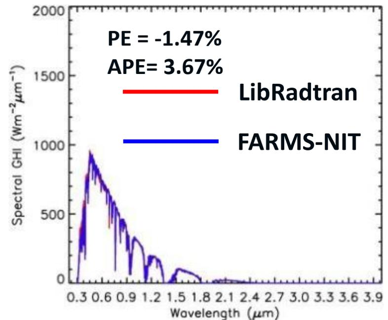
Spectral GHI for US standard atmosphere 1976 when  $\theta_0=30^\circ$ ,  $\tau=10$ ,  $De=20\mu\text{m}$ , and surface albedo=0.0. (**red: simulation by LibRadtran**; **blue: FARMS-NIT**)
