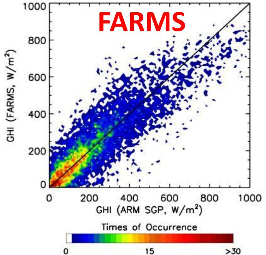
**GOES satellite data is collocated to ARM SGP site. The satellite-based retrievals of cloud properties are used as inputs to the two-stream RRTMG(used in meteorological applications) and FARMS. A total number of 9669 scenarios associated with cloudy-sky are selected during 2009-2012.**
