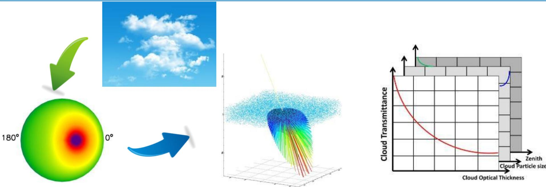
A lookup table of cloud transmittance using the LibRadtran model is computed for **2002 wavelengths**, **39** cloud optical thicknesses, **28** cloud effective particle sizes, **50** solar zenith angles, **25 viewing zenith angles** and **18 relative azimuth angles**.
