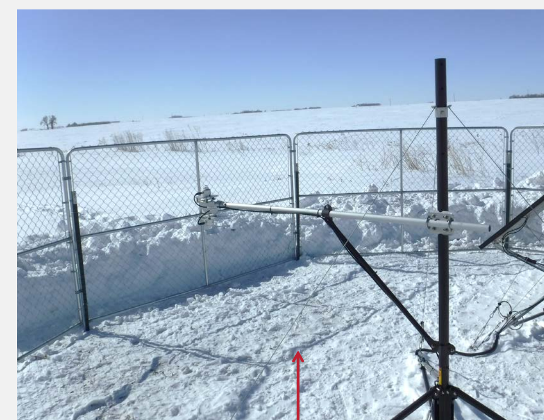
Influence of repeated fresh snow events on albedo measurements. Consider: (1) upward pyranometer condition, and (2) direct correlation with PV snow loss due to accumulation on PV arrays.
