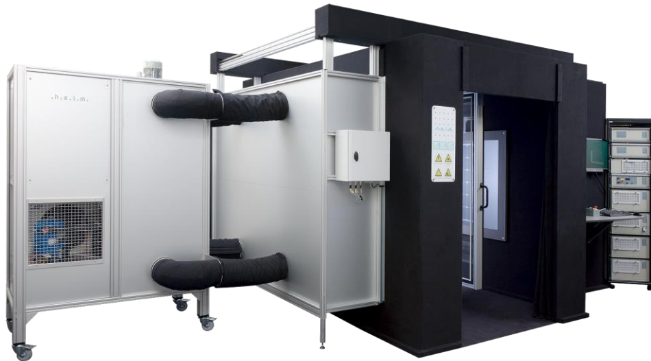
Fig. 4.3.1 Class AAA solar simulator from h.a.l.m. used at CFV
