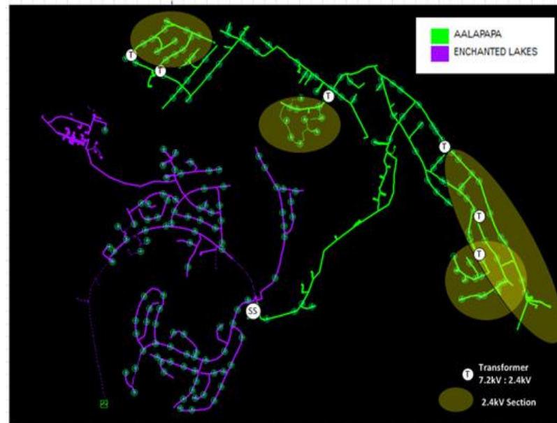
Substation A: Feeder Model
