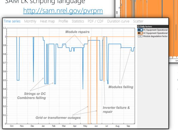
Samples failure distributions for components in a PV system and predicts failure times, replacement costs, and performance/cost impacts for a more realistic representation of LCOE of PV systems
