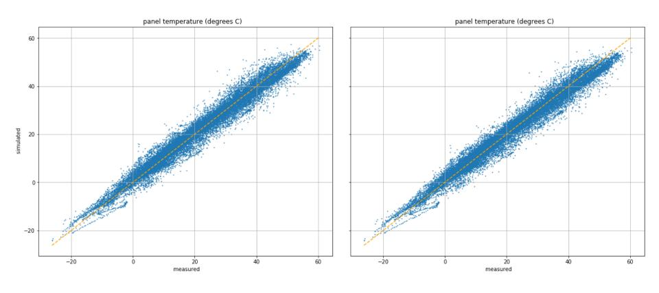
Heat loss factor = 29 W/m<sup>2</sup>/K MBE = 0.3 °C RMSE = 2.8 °C Heat loss factor = 29.9 W/m<sup>2</sup>/K MBE = 0.0 °C RMSE = 2.8 °C
