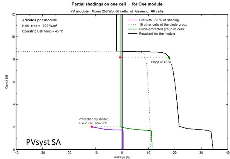
By-pass diodes: derive the current in this sub-module
