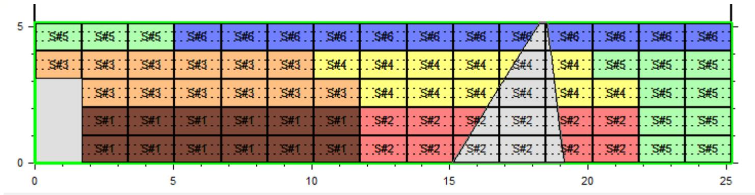
**Linear Shading Factor** = Nb of shaded sub-modules / Total nb. of sub-modules
