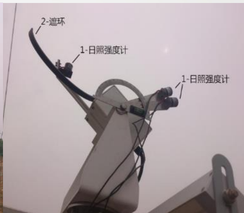
遮环以及日照传感强度计 Occlusion ring and sunshine sensor intensity meter
