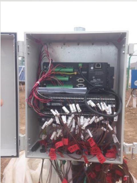
温度采集系统 Temperature acquisition system
