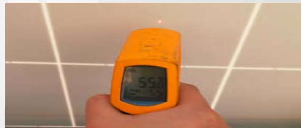
组件背板测温 Component back panel temperature measurement
