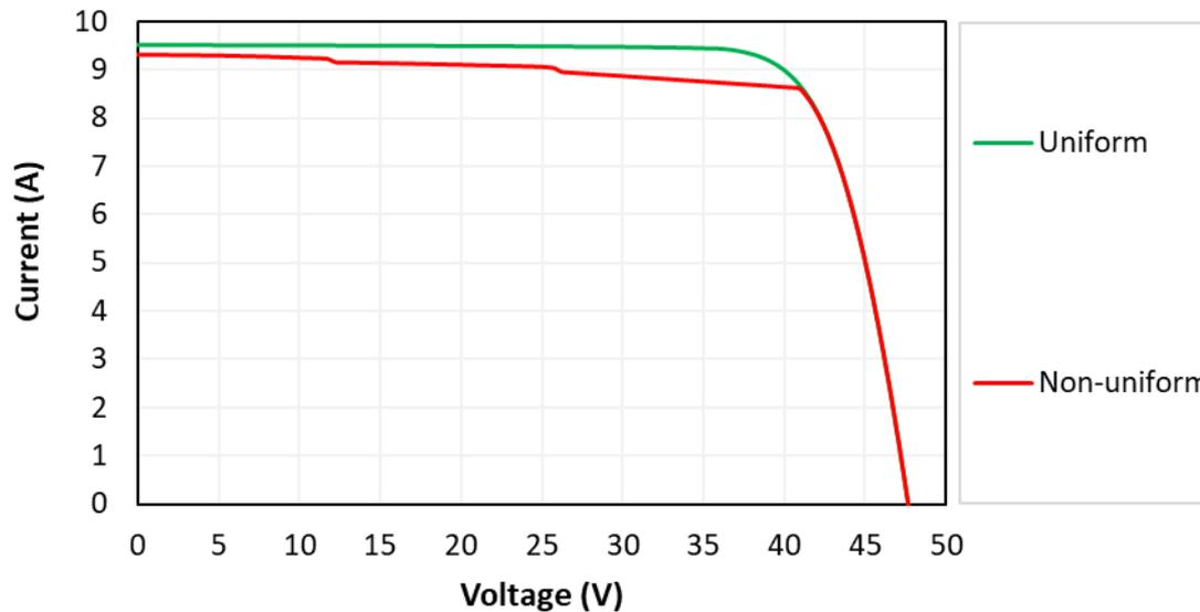
**Significant cell-to-cell mismatch loss**
