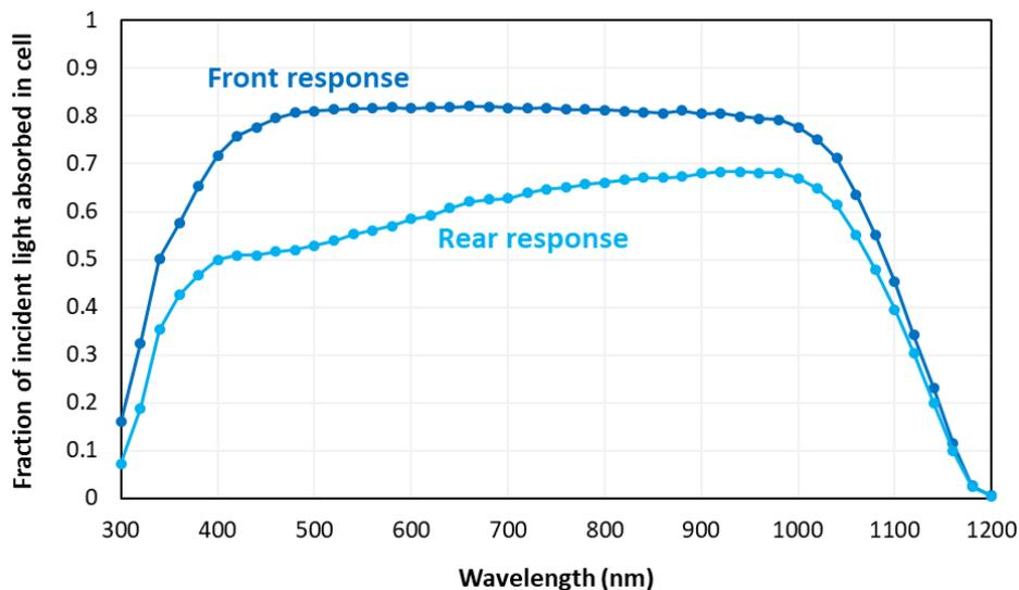
As simulated by PV Lighthouse for contemporary bifacial module under normal incidence.
