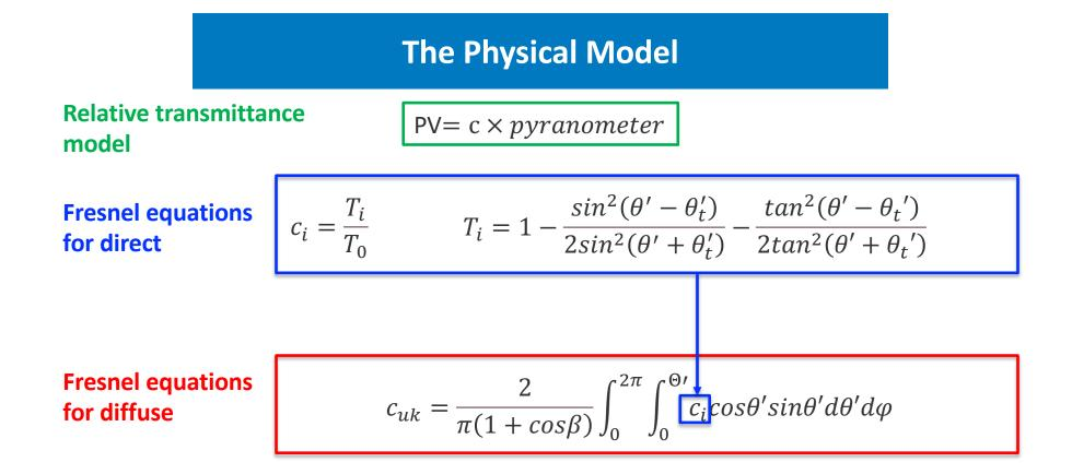
The physical models use the Fresnel equations to analytically solve the beam transmission through the instrument covers. The transmission of diffuse radiation is computed by integrating the Fresnel equations over the PV surfaces.
