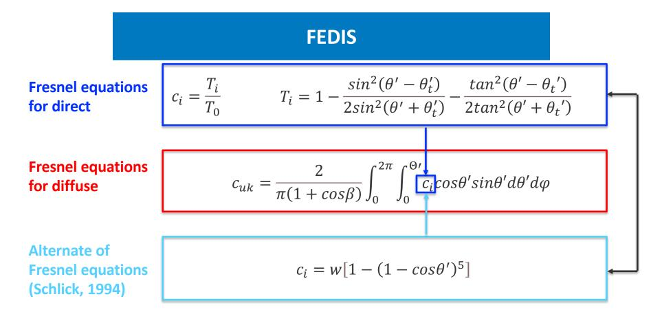
Given an alternate form of the Fresnel equations initially proposed by Schlick and adopted by extensive applications for direct radiation, the space integration of transmittance can be analytically solved for inclined PV surfaces.
