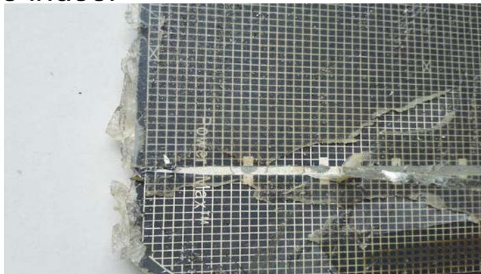
Structure of electron connection in front surface and back surface
