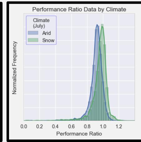
**Above:** The probability distribution of performance ratio can vary by panel manufacturer or climate type at different times of year. Thus, a generalized quantile regression model can reproduce the annualized performance ratio probability density function for any given site.
