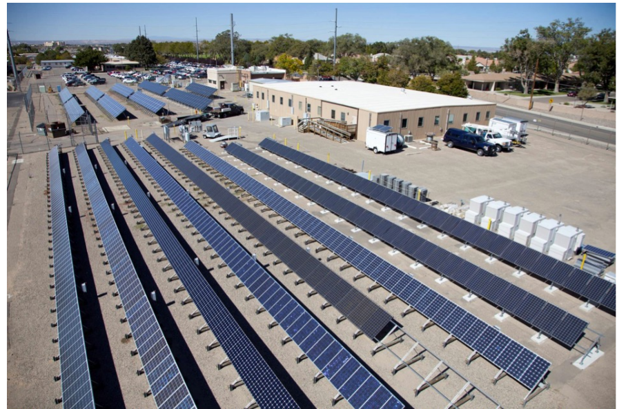
Test beds at Sandia National Laboratories Photovoltaic Systems Evaluation Laboratory (PSEL) in Albuquerque, New Mexico
