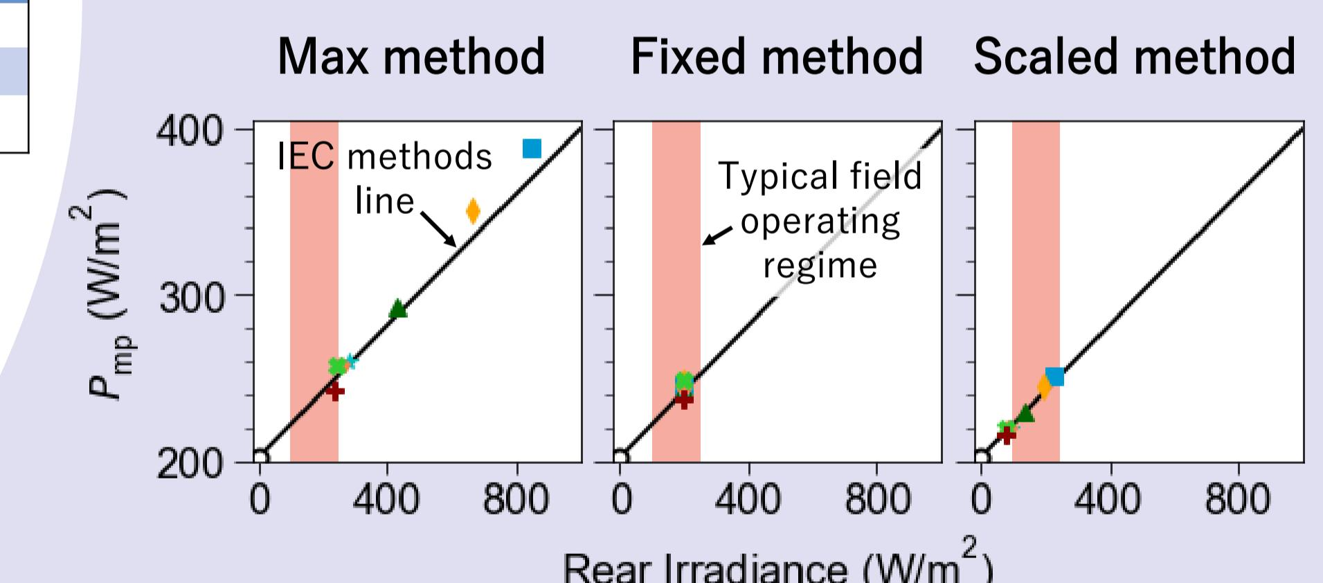
Scaled method reduces rear incident irradiance to levels typical during field operation
