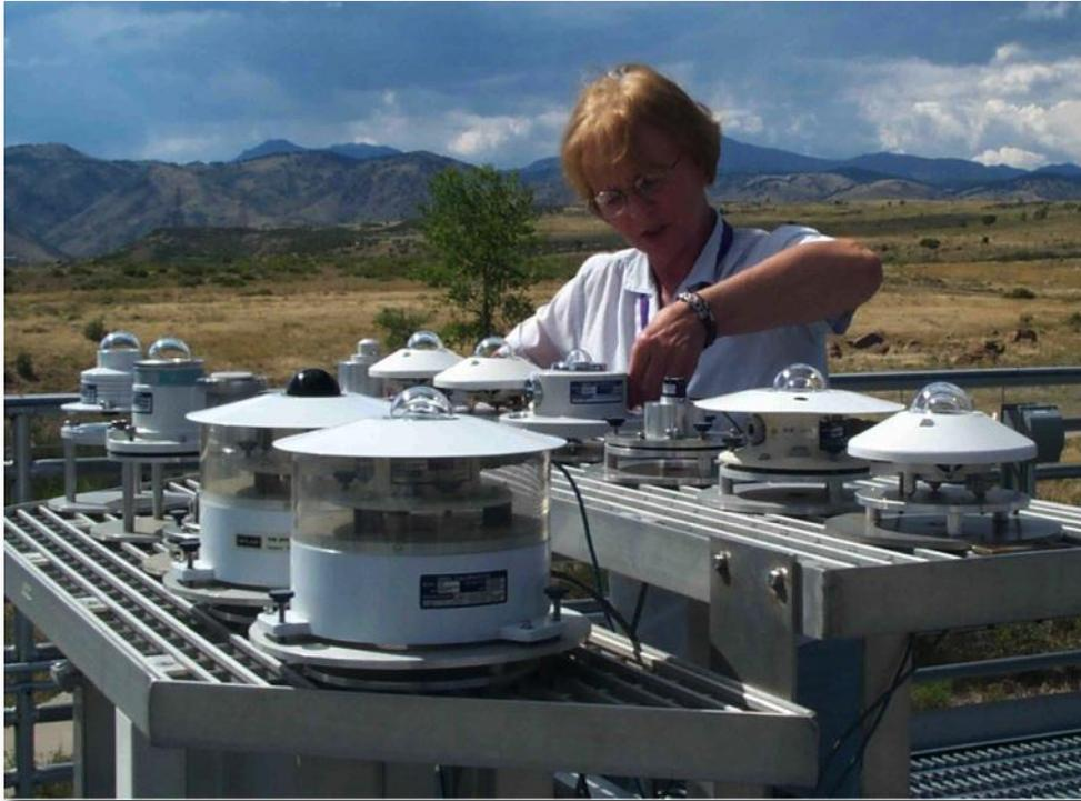
*Pyranometers with Ventilators*
