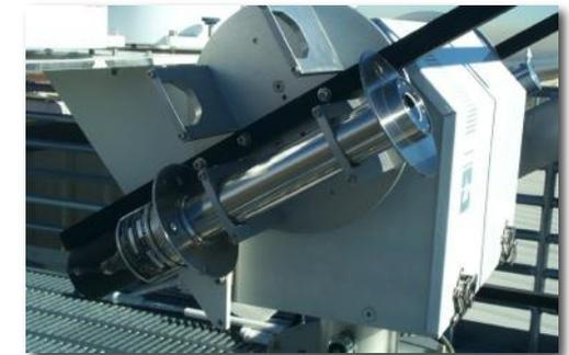
**Normal Incidence Pyrhelioscope (NIP)**
