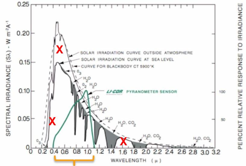
Typical photodiode detector (left) and spectral response of LI-COR pyranometer (right).
