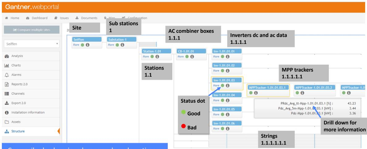
Can easily check various losses such as downtime, mismatch, shading, tracking per component ...
