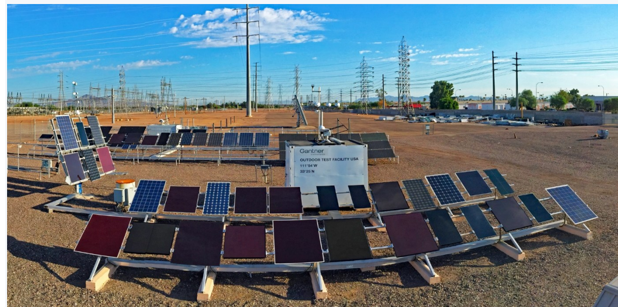
Outdoor Test Facility Solution 30 Channels, Gantner Instruments Research site, Arizona
