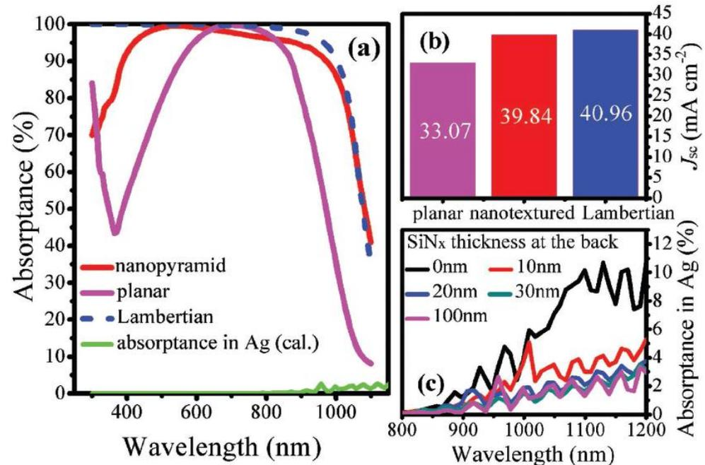
Applying the all-solution-processed nanopyramids to ultrathin c-Si (30μm), near-Lambertian light trapping effect is achieved, the calculated  $J_{sc}$  is far higher than that of the planar c-Si.
