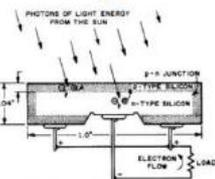
Fig. 3. Schematic of early silicon solar cell [6].
