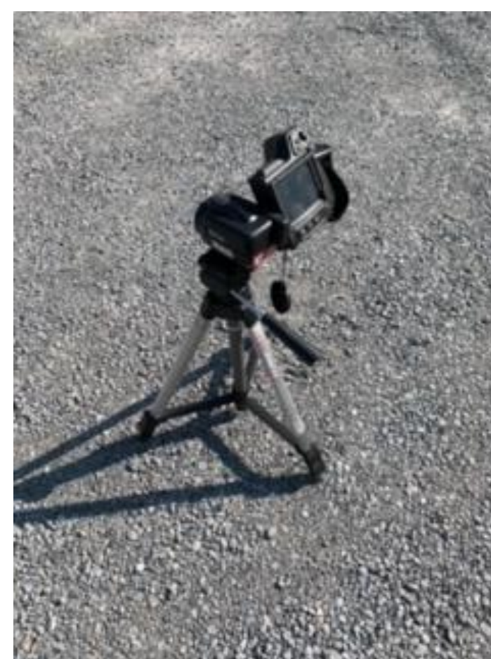
Figure 4: Thermal Camera used to collect panel temperature.
