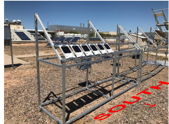
NOCT testing at ASU-PRL
