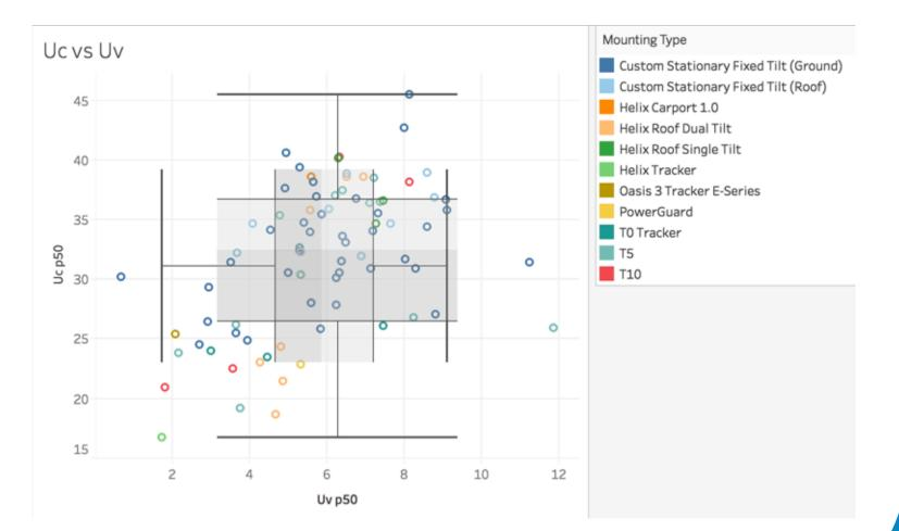
• Greater sensitivity to wind speed measured at array height than when measured at 10m
