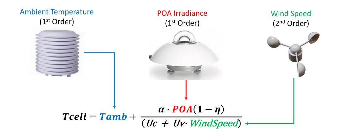
Uc: Constant Component (insensitive to wind speed)Uv: Wind speed sensitivity
