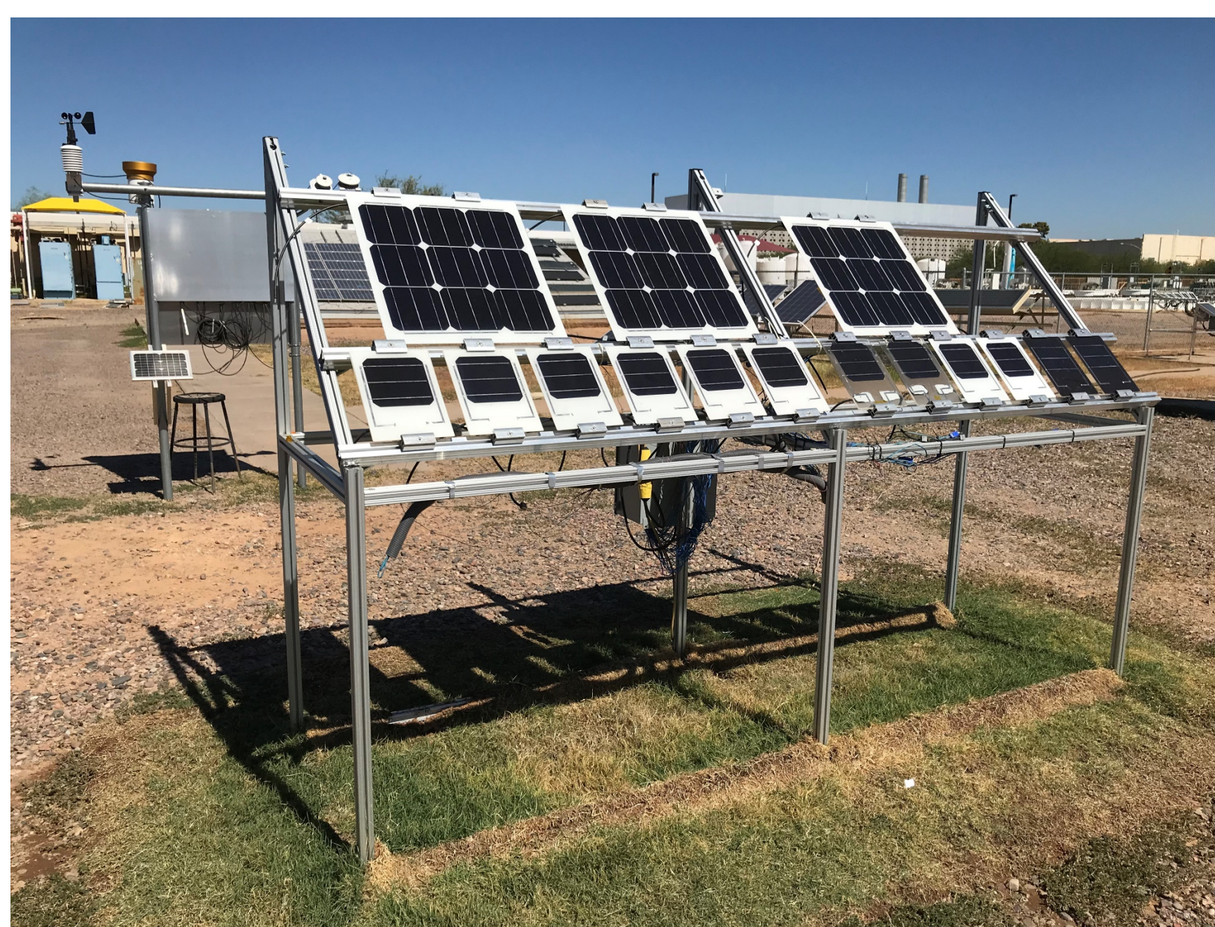
Fig. 2. A photo of 1-cell and 9-cell modules installed at open rack mount for thermal testing at Mesa, Arizona.
