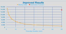
Comparison of inverter clipping estimated using 1 hour time-step with steady state using time step durations of 1, 2, 3, 5, 6, 10, 12, 15, 20, 30 minutes and 1 hour. Example is for 1,176 kW PV system with 900 kW inverter using weather data from Oahu, Hawaii. Results generated using HOMER Pro Version 3.14.5
