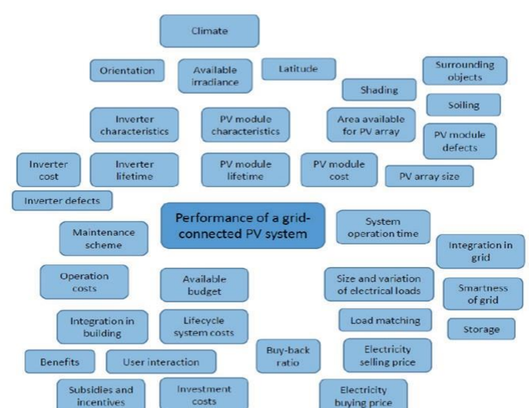
Figure 3: Key factors that determine the optimal performance of PV systems.
