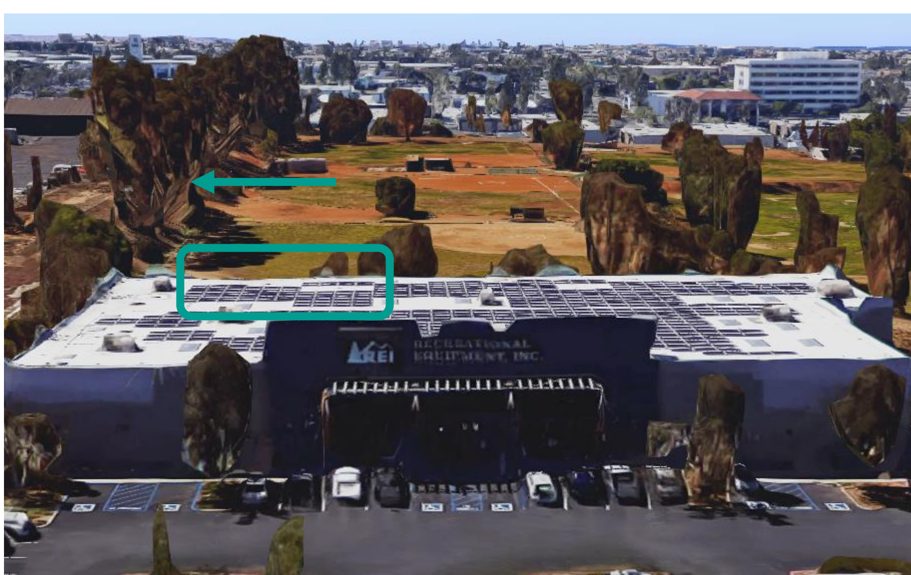
Figure 1: REI San Diego location with shading trees indicated with an arrow and PV modules affected by those trees marked with a rectangle.
