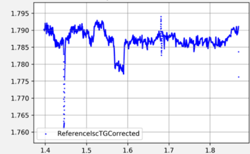
2A2 Reference Module Temperature+Irradiance Corrected Isc vs Airmass
