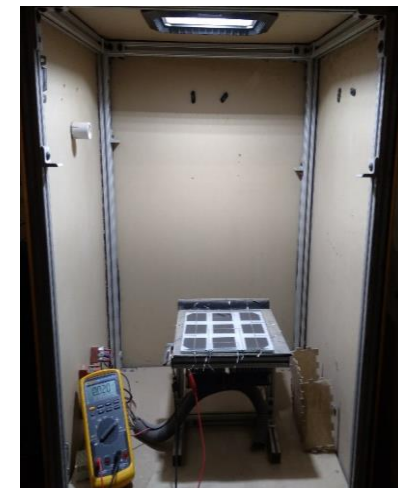
In-situ Soiling Uniformity ( I_{sc} ) Measurement
