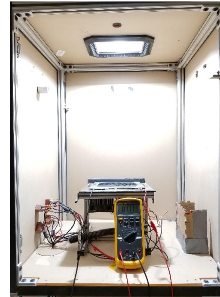
In-situ Transmittance ( I_{sc} ) Measurement
